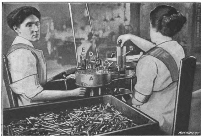
Fig. 9. Cartridge Clipping Machine—Assembling the Cartridges in the Clip
