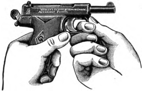
FIG. 1.—Showing the position of the hands for drawing out the trigger guard.
