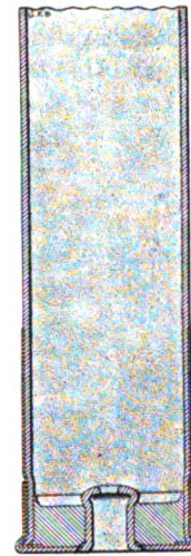
FIG. 32.—THE "U.M.C. TRAP" CASE.
