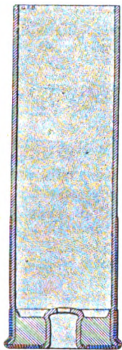
FIG. 28.—THE "E.B.L." OR HALF-BRASS CASE.
