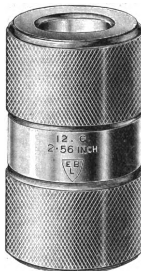
SOCKET GAUGE MADE BY MESSRS. ELEY BROS. TO THE STANDARD MINIMUM GUN CHAMBER SIZES.
